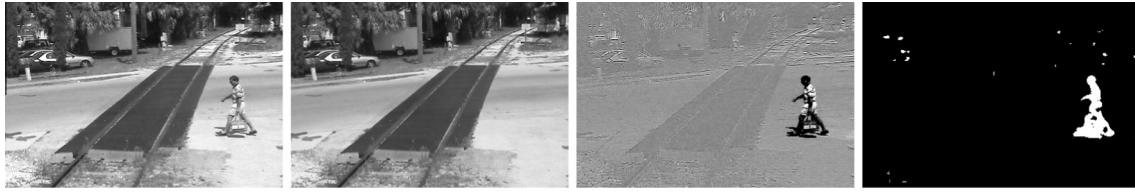
Fig. 1. First Row: Original image (309), low-rank matrix L (background), Second Row: Sparse matrix S (foreground), foreground mask.
